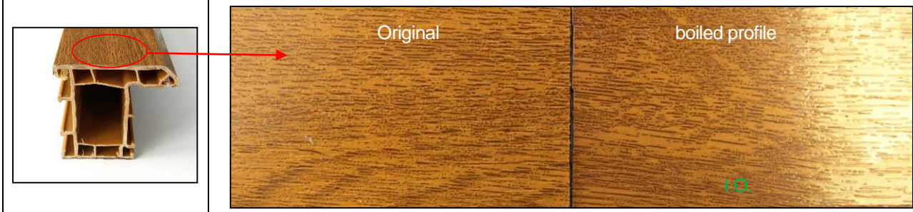
Picture 1 – Boil test according to AMMA 303-18 – Comparison (Original – Boiled profile)
